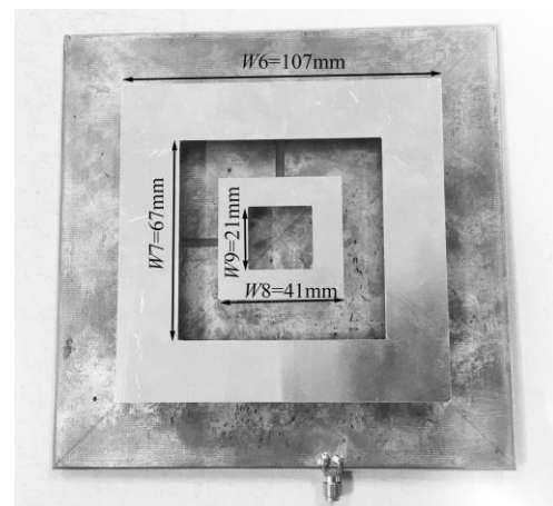
Figure 5. Photograph of the fabricated antenna
